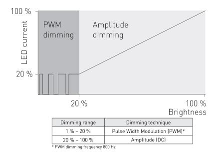
Helvar hybrid dimming products combine the best features from Amplitude dimming and from Pulse Width Modulation (PWM) dimming. CCR is a very efficient technique for dimming the light output especially on higher range. On lower range, the hybrid dimming products implement high-frequency PWM dimming to ensure high quality dimming from 20 % down to 1 % providing low flicker dimming perfor-
